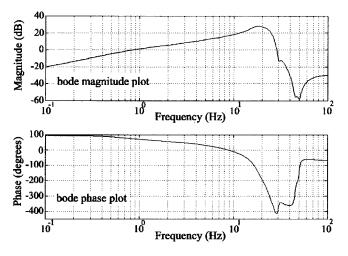
FIG. 3. Bode magnitude and phase plots illustrating the open loop response of the controller. The controller contains a high pass corner filter 0.7 Hz; transitional differentiator 0.35-0.8 Hz; transitional differentiator 2-14 Hz; two pole low pass 18 Hz, Q=3, notch 30 Hz; two pole low pass 24 Hz, Q=4, notch-45 Hz; two pole low pass 28 Hz, Q=5, notch=50 Hz and a simple low pass at 14 Hz.
