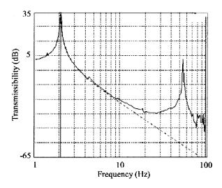
FIG. 5. Vertical transfer function of the prototype set of upper blade springs (illustrating nonideal behavior). The solid trace is the experimental transfer function and the dotted trace is the theoretical transfer function for an ideal massless spring with the same parameters. The first internal resonance is at  $\sim$ 55 Hz.
