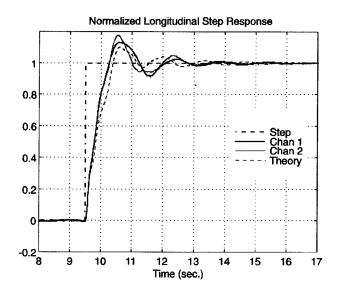
FIG. 6. Longitudinal step responses for the two longitudinal actuators (channels 1 and 2) compared to the theoretical prediction from a MATLAB model.
