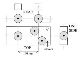
FIG. 2. Schematic view of the upper mass showing the locations of the actuator coils with respect to the mass. The two coils (numbered 1 and 2) acting on the rear of the mass control the longitudinal and rotational modes, three coils acting on the top control tilt, vertical and roll, and the one on the side controls the sideways motion. The coils are rigidly attached to the damping arm (see Fig. 1).
