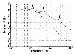
FIG. 8. Theoretical MATLAB plots of the vertical (solid trace) and horizontal (dotted trace) transfer functions for the GEO 600 triple pendulum suspension. the flattening of the vertical transfer function due to the nonideal nature of the cantilever blades is included in the model. The horizontal transfer function is calculated from the top point of the suspension to 1 mm above the center of mass of the test mass.
