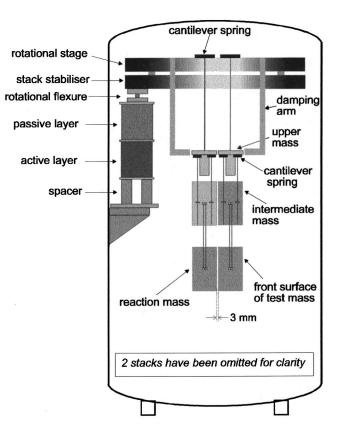
FIG. 1. Schematic of the overall main suspension (viewed perpendicular to the optic axis). A reaction pendulum, which is used to apply global feedback forces to the main pendulum, is shown adjacent to the main pendulum.
