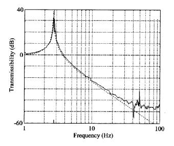
FIG. 7. Vertical transfer function of the redesigned set of upper blade springs (illustrating more closely ideal behavior). The solid trace is the experimental transfer function and the dotted trace is the theoretical transfer function for an ideal massless spring with the same blade parameters. The notch at 40 Hz is associated with a structural resonance in the measurement system. The peak near 50 Hz is due to electrical mains interference.
