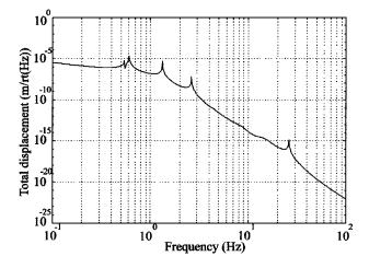
FIG. 9. A theoretical MATLAB plot of the total displacement noise of the test mass, which was calculated from transfer functions of triple pendulum and stack, in both vertical and horizontal dimensions, and incorporates a typical seismic noise input.
