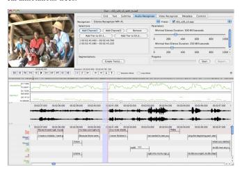
**Figure 1.** Use of a silence detector in ELAN 3.6: Detector parameters can be adjusted on the right side. A video viewer is on the left side. Results will be added as a new tier to the annotations and waveforms at the bottom.
