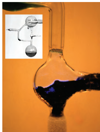
Figure 5. Blue anthracene fluorescence as chemiluminescence from a reaction between anthracene- \text{Na}^+ and \text{TMPD}^+\text{ClO}_4^- in 1,2-dimethoxyethane. The fluorescence originates by triplet-triplet annihilation from the initially produced anthracene triplets. Insert: the evacuated pyrex chemiluminescence cell.
