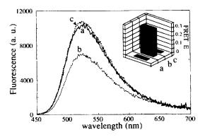
FIGURE 5 Lucifer Yellow fluorescence of LY-BIPS before (a) and after (b) lightinduced conversion of spiropyran to merocyanine. After 1 h at room temperature, the molecule reverted to the spiropyran form, as evidenced by the restoration of the fluorescence to its original value (c). Inset: corresponding FRET efficiency values.
