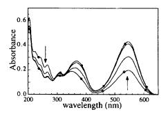
FIGURE 2 The photochemical conversion from the spiropyran to the merocyanine form as a function of the duration of UV irradiation. Absorption spectrum after a 2 min (O) and 15 min ( $\bullet$ ) exposure to UV (254 nm) are depicted. The arrows indicate the decrease in the spiropyran form or the increase in the merocyanine form. The initial spiropyran state is not shown (see Figure 4A).
