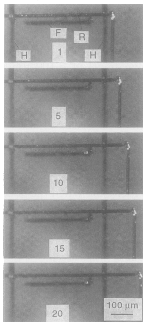
Fig. 6. Front view of the linear micromotor after 1, 5, 10, 15, and 20 cycles. The horizontal bar is moved \sim 100 \mu\text{m} to the right during 20 cycles (H, holders; F, fork; and R, rod).
