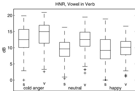
Fig. 2. Results of the statistical analysis of the estimated HNR for vowels from the sentence final verb and the three emotional states. For each case the box ranges from the lower to the upper quartile with the median value indicated by a line, and the total range indicated by the whiskers. Outliers are indicated by crosses. For each emotional state higher HNR is found when the verb is accented (case 'v').
