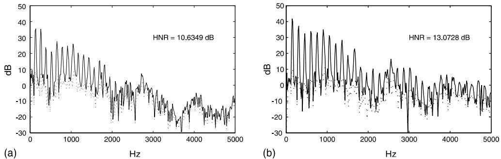
Fig. 1. Spectra of the original signal (—) and the estimated noise component (· · ·) for the vowel /a/ in the sentence final verb for neutral emotional state and (a) accentuation on the NP, (b) accentuation on the sentence final verb, corresponding to *neutral case 's'* versus *neutral case 'v'* in Fig. 2.
