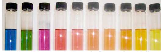
Figure 2.1: Colloidal solutions of silver, gold and bimetallic nano-particles(Au-Ag)[23]. Depending on the actual size or composition, the energy position of the plasmonic excitation can be tuned within a large spectral range.
