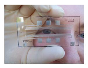
Figure 1: Photograph of the molecule chip, held by one of us (S.A.M.). The array of 1254, 10 µm diameter and 4 mm long electrodes extends over a total length of 50 mm. The electrodes run vertically, and are connected to either one of the six macroscopic pads to which the sinusoidal voltages are applied. (Photograph by Dr. Cynthia E. Heiner, FHI).
