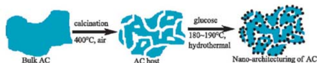
Scheme 1. Nanoarchitecturing of activated carbon by anchoring nanostructured carbon spheres onto the AC host.
