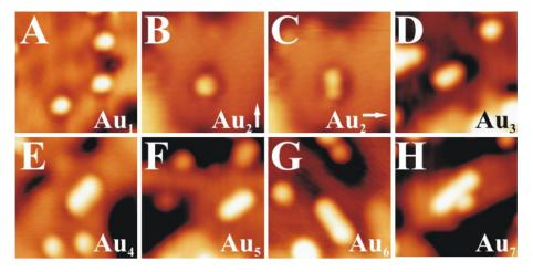
**Fig. 2** (Color online): STM topographic images of **(A)** Au monomers, **(B,C)** upright and flat Au dimers and **(D-H)** Au chains containing three to seven atoms on MgO / Ag(001) (-0.4 V, 5×5 nm<sup>2</sup>).
