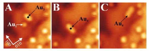
**Fig. 4.** (Color online): **(A)** STM image showing a trimer and monomers on the MgO film. A +2V bias pulse was applied to the trimer at the position marked by the black dot, creating a tetramer chain **(B)**. The same manipulation procedure was repeated for the tetramer **(C)**, inducing the diffusion of the adchain.
