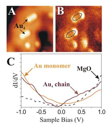
**Fig. 3** (Color online): **(A)** Topographic and **(B)** differential conductance image of two Au<sub>4</sub> chains on MgO / Ag(001) (-0.4 V,  $6.5\times6.5$  nm<sup>2</sup>). **(C)** dI/dV spectra of a monomer and an Au<sub>4</sub> chain (setpoint bias +0.8 V). Apart from the end-states, no dI/dV features are visible in spectroscopy within the accessible bias window.
