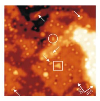
**Fig. 1** (Color online): STM topographic image of Au adatoms and clusters on a 2 ML thick MgO film on Ag(001) (-0.4 V,  $19\times19$  nm<sup>2</sup>). The arrows mark [100] and [010] oriented Au chains, while the circle depicts a chain in [110] direction. The squares frame two triangular 2D clusters.
