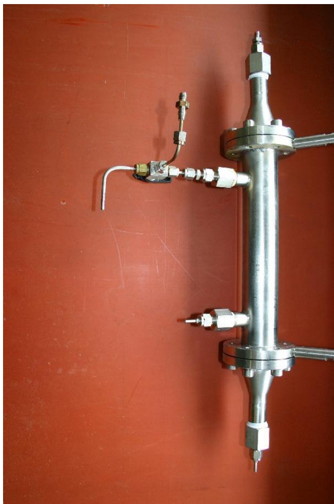
Figure 2.2.11: Configuration of membrane module with feed inlet in shell site (left picture in figure 8). The three ways valve in the feed inlet allowed to switch the feed either in shell site of membrane module or a direct feed to the GC.
