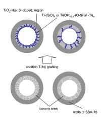
micropores are located in the corona of SBA-15 channels, this reaction leads to the formation of  $TiO_2$ -like nanoareas with dimensions of around 1-2 nm. The reaction of Ti with the silica leads to the elimination of surface defects and of the regions with high hydroxyl density, with a better ordering and an intensification of the XRD reflections at small angles.
