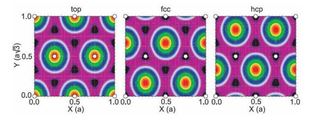
FIG. 4: (Color online) Fourier terms for the interaction of an atom with a fcc(111) surface. In (a) the top-term  $f_{top}$ , in (b) the fcc-term  $f_{fcc}$ , and in (c) the hcp-term  $f_{hcp}$ , defined in Eqs. (3 - 5) respectively, are shown as a function of x and y in units of the lattice constant a. In all three figures the white circles represent the position of the first layer substrate atoms.
