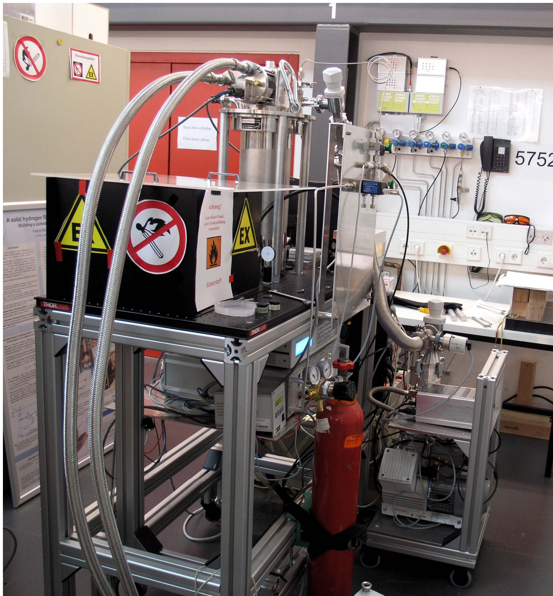
Figure 3-7: The entire setup with vacuum system on the right, gas inlet system, and temperature controller.
