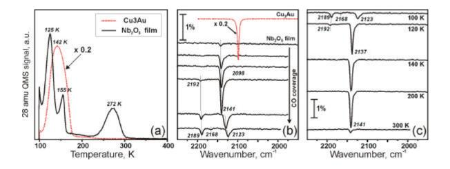
Fig. 2. (a) Typical TPD spectrum of CO adsorbed on thin niobia films at 100 K. (b) IRAS spectra of CO adsorbed on thin niobia films as a function of CO exposure at 100 K. (c) IRAS spectra of CO adsorbed at 100 K and subsequently flashed to the indicated temperatures. All spectra are recorded at 100 K. The TPD and IRAS spectra for a
