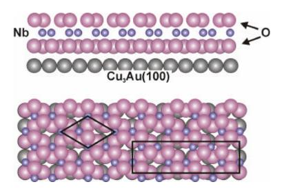
Fig. 1. Cross and top views of the thin niobia film grown on  $Cu_3Au(100)$ . The unit cell of niobia overlayer is indicated as a rhomb. The rectangle shows the (2x7) coincidence superstructure, which is formed between oxide and metal substrate lattices. The surface shows a hexagonal lattice with a 5.3 Å periodicity.
