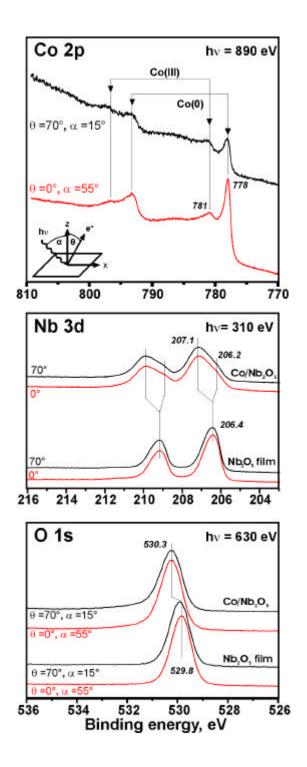
Fig. 5. Co2p, Nb3d and O1s regions of photoelectron spectra measured at two different geometries as depicted in the inset. The spectra for Nb and O core levels are shown before and after 2 Å of Co have been deposited at 300 K.
