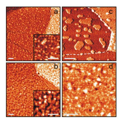
Fig. 3. STM images of Co deposited at 300 K on thin niobia films. The Co coverage is 0.5 Å (a,c) and 2 Å (b,d). Images (c) and (d) are taken after heating the same samples to 500 K. The scale bar corresponds to 20 nm. Tunneling parameters are (a) bias 1.2 V, current 1 nA; (b) 0.75 V, 0.7 nA; (c) 1.25 V, 1.3 nA; (d) 0.75 V, 1 nA. Image (c) is presented in differentiated contrast, where the domain boundary is marked by the dash line.
