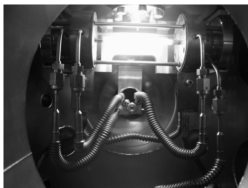
Figure 6: Catalytic wall reactor in operation, T = 1250\text{ }^{\circ}\text{C}
