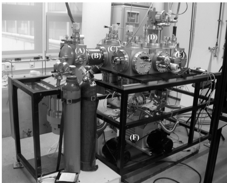
Figure C-2 Tandem mass spectrometer in the FUB lab without any cables connected. From left to right one can see the source chamber (A), bellow (B), high vacuum chamber (C), cryostat (D), detector region (E), and foreline pumps (F).
