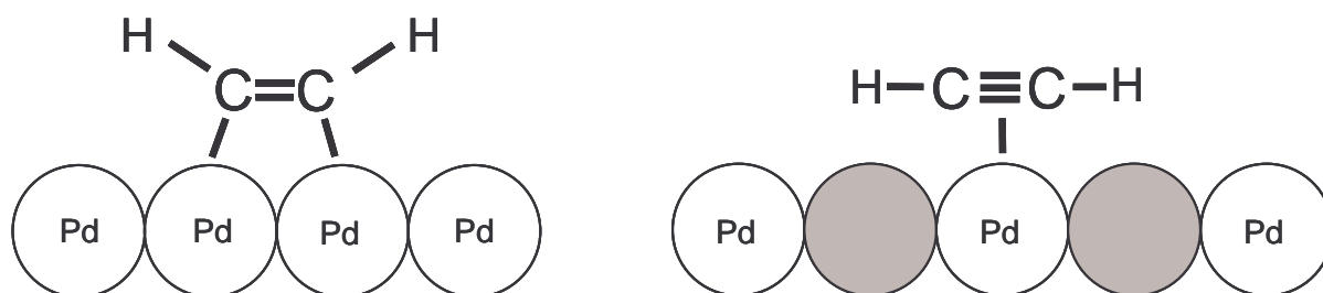
Figure 1: Di- \sigma bonded acetylene molecule to two neighbouring Pd atoms (left) and a weakly \pi -bonded acetylene molecule to an isolated Pd atom (right). Only the \pi -bonded acetylene is hydrogenated in high selectivity to ethylene.
