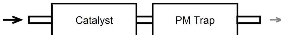
Fig. 2.3: Catalyst-filter-combination used for exhaust treatment. The aim is to oxidize \text{NO}_x to \text{NO}_2 and to regenerate with this oxidant the soot trapped in the filter device.
