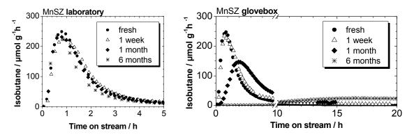
The storage conditions (temperature, O<sub>2</sub> and H<sub>2</sub>O partial pressure) can influence the performance of sulphated zirconia catalysts. Through variation of the conditions different materials can be generated from the same parent compound. Such samples provide a unique opportunity to identify properties that are relevant for activity.
