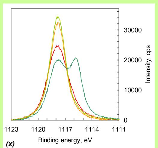
XPS investigation of PdGa and Pd<sub>3</sub>Ga<sub>7</sub> shows Ga<sub>2</sub>O<sub>3</sub> at the surface which could not be significantly by hydrogen treatment at elevated reduced temperature.
