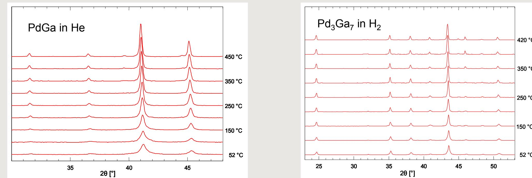
In situ XRD measurements were conducted using a STOE diffractometer with Cu-Kα radiation in Bragg-Brentano geometry (secondary monochromator) equipped with a Bühl HDK chamber.
