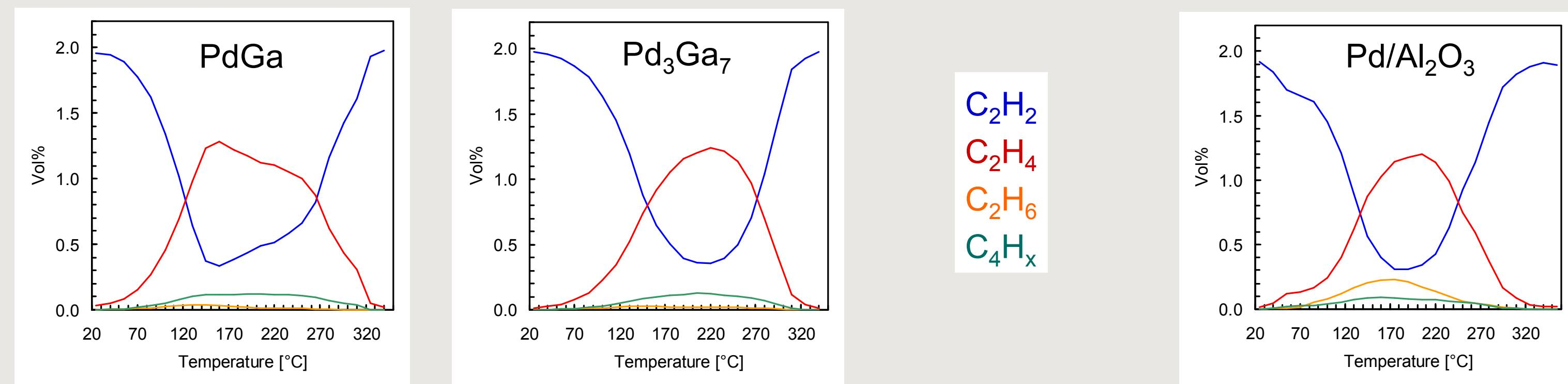
Catalysis studies were performed in a plug flow reactor (C<sub>2</sub>H<sub>2</sub> / H<sub>2</sub> ratio 1:2, total flow 30 ml/min) with gas phase analysis using MicroGC Varian CP4900. The amount of catalyst was PdGa (50 mg), Pd<sub>3</sub>Ga<sub>7</sub> (100 mg) and reference Pd/Al<sub>2</sub>O<sub>3</sub> (0.5 mg, 5 wt%). The red curve shows the concentration of the product ethylene, yellow shows the total hydrogenated ethane and green the dimerisation products.
