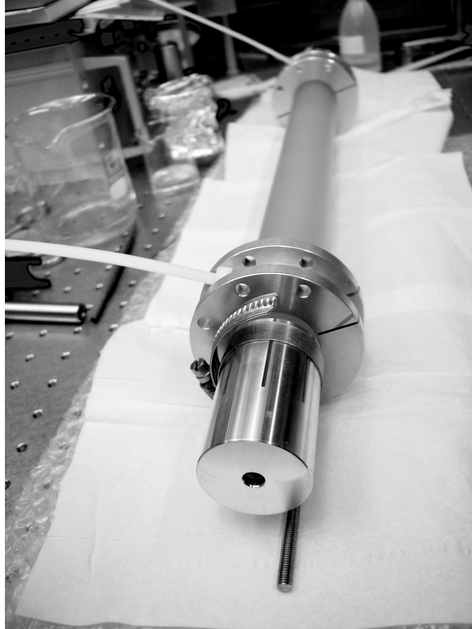
Figure 2.9: Picture of the confocal interferometer.
