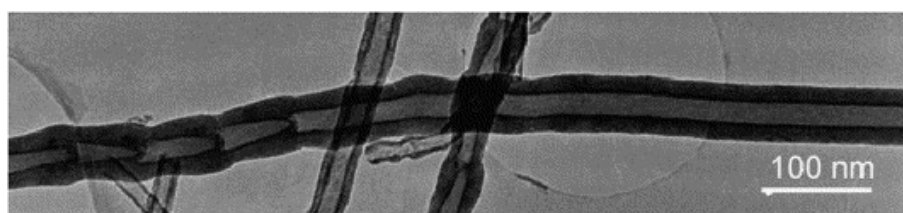
Fig. 5. TEM image of a special tube (the thwart one) constructed by half of a normal tube with a long hollow channel and half of a bamboo-shape tube with partitioned small hollow compartments.
