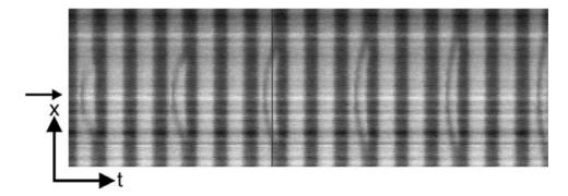
**Figure 4.** Space–time plot (380  $\mu$ m × 11.1 s) for the measurement displayed in figure 2(a) taken along a cut through the laser's path (indicated by the small black arrow). The start of the dark phase of the homogeneous oscillation is marked in one place by a thin vertical line in order to show the phase delay caused by the emitted wave.
