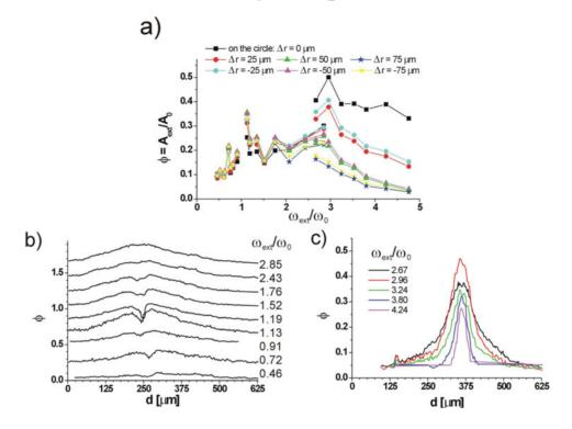
**Figure 10.** (a) Ratio  $\phi = A_{ext}/A_0$  for different distances from the laser's path depending on  $\omega_{ext}/\omega_0$ . (b)  $\phi(x)$  for measurements close to  $\omega_{ext}/\omega_0 = 1$ . The curves have been shifted with respect to each other for better viewing. (c)  $\phi(x)$  for measurements for  $\omega_{ext}/\omega_0 > 1$ .
