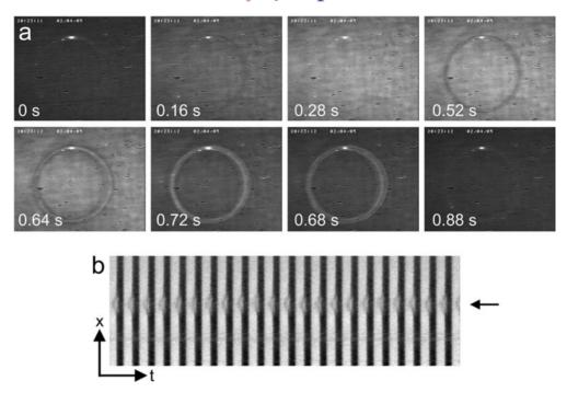
**Figure 6.** (a) Sequence covering one period of the global oscillations. (b) Spacetime plot (430  $\mu$ m × 21 s) taken along a cut through the laser's path (marked by the black arrow). Parameters:  $\omega_{ext} = 8.78\omega_0$ , T = 535 K,  $p_{CO} = 8.9 \times 10^{-5}$  mbar,  $p_{O_2} = 3.0 \times 10^{-4}$  mbar.
