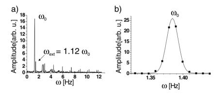
**Figure 8.** Two spectra measured directly on the laser's path. (a)  $\omega_{ext} = 1.12\omega_0$ , (b)  $\omega_{ext} = 0.99\omega_0$ . In (a) both frequencies  $\omega_{ext}$  and  $\omega_0$  are detected, while (b) only shows the region close to  $\omega_{ext} = \omega_0$ . The resolution of the spectrum is not sufficient to differentiate between  $\omega_{ext}$  and  $\omega_0$ .
