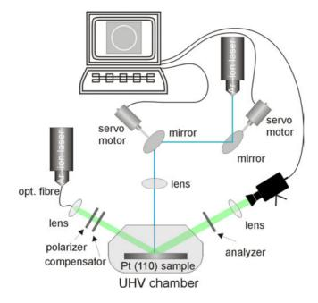
**Figure 1.** Sketch of the experimental set-up. The green beam path shows the EMSI, while the blue beam path shows the set-up for the heating laser. The laser beam positioning mirrors are mounted perpendicular to each other, and are controlled by computer utilizing servomotors.
