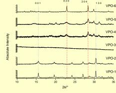
The ED and XRD patterns for VPO-1 and VPO-2 show VOHPO<sub>4</sub>·0.5H<sub>2</sub>O phase, VPO-4, VPO-5 and VPO-6 show  $(VO)_2P_2O_7$  phase.
