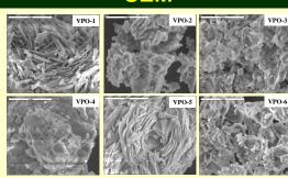
The particle size becomes smaller (VPO-2 and VPO-3) and agglomeration occurs as milling time increases (VPO-4). Mechanotreated samples showed more rounded particles compared with VPO-1, which showed needle like particles. VPO-5 after heating in vacuum revealed a similar morphology as VPO-1.
