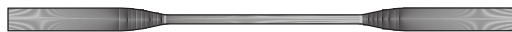
Figure 4.1: In a first pull extension the so-called neck is produced. The neck defines the shape of the tapered fiber ends, which is of relevance for the welding.
