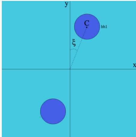
Figure 2.3: The drift-correct method. The centroid C of one of the black holes is tracked, the angle \xi measured, the effective angular velocity of the centroid \Omega_c is computed, and the shift vector is changed according to Eq. (2.46).
