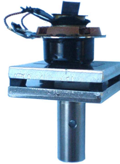
Figure 4.7: Laser shutter. A small loudspeaker is used to move the beam shutter. It is mounted on two aluminum plates which are connected by damping material in order to minimize noise transfer to the optical table.
