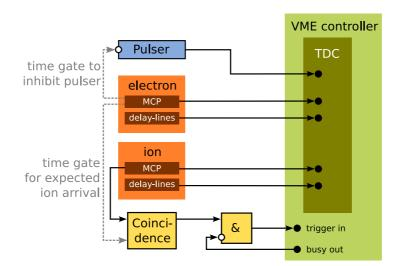
Figure 3.7: Scheme of our data acquisition system.
