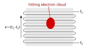
Figure 3.5: Working principle of a delay-line anode.  $t_1$  and  $t_2$  are the signal propagation times of the electron cloud to either end of the wire. The difference is proportional to the position along the x coordinate. For two-dimensional information at least two layers are necessary.
