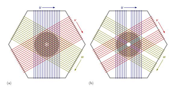
Figure 3.6: Design of the hexagonal anodes used as (a) electron detector, (b) ion detector. The grey disks represent the areas covered by the MCPs and, hence, the active detection regions.
