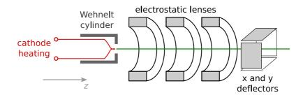
Figure 3.1: Schematic drawing of our electron gun. All lenses, the cathode and the Wehnelt cylinder can be set on arbitrary potentials. One of each pair of deflector plates is grounded, while the other one is on adjustable potential.
