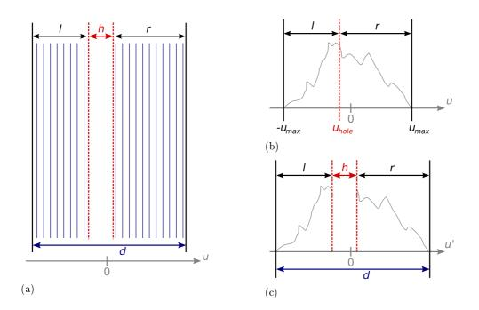
Figure 4.5: Reconstruction of the hole in the distribution of position signals: (a) design of a hole-containing delay-line layer, (b) sample distribution of raw signals before and (c) after insertion of the hole.
