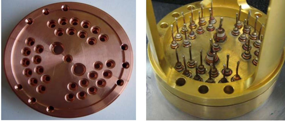
Figure 4.14: Mounting flange of the UHV trap chamber. The machined piece is shown on the left, the gold-plated and with 33 electric feedthroughs equipped mounting flange with the adjacent workpiece on the right side.
