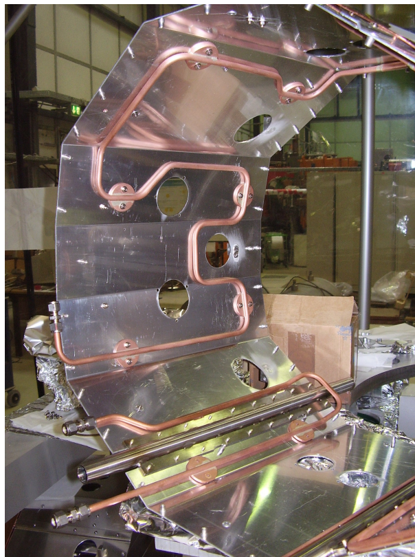
Figure 3.16: Water cooling pipes on the 80K radiation shields to protect the multi-layer insulation during the bake-out
