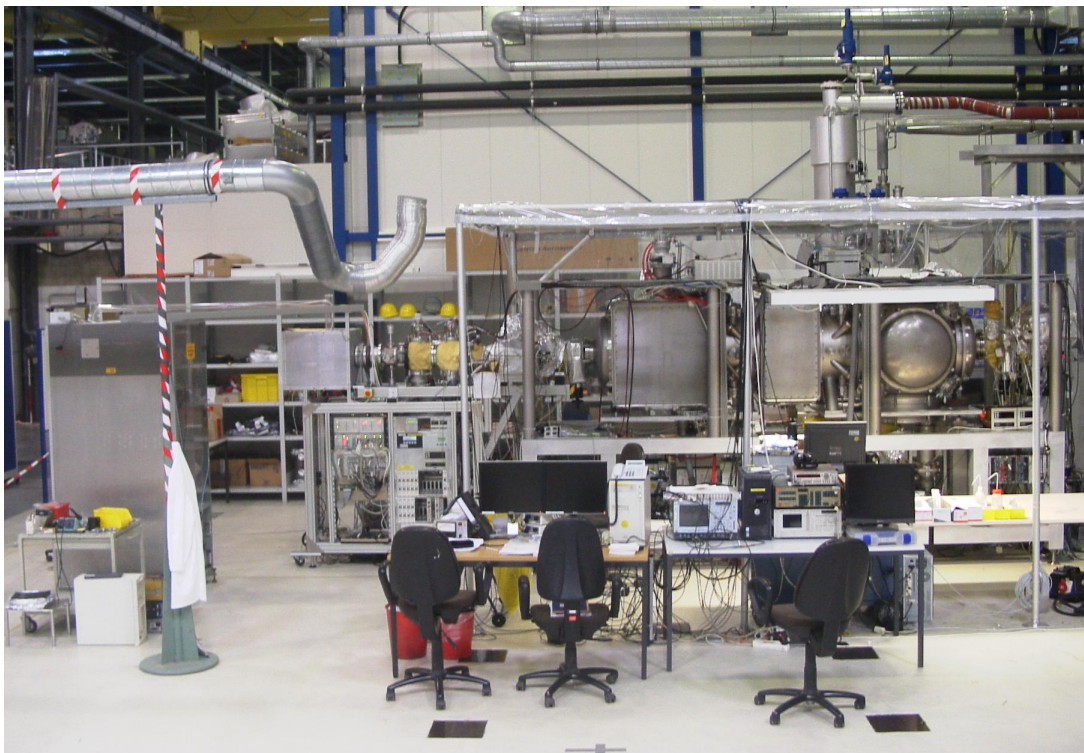
Figure 3.1: Overview of the CTF with the ion source and injection line on the left and a part of the helium refrigeration system in the background
