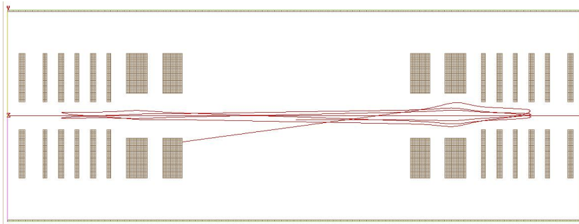
Figure C.2: Unstable trajectory of one N_2^+ ion with 7.1 keV energy simulated with SIMION
