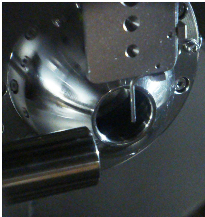
Figure 3.13: Photograph taken looking into the target chamber. The tip of the gas injection capillary is shown in the centre of the image, entering from above. The capillary is mounted below a steel plate with varying known hole sizes, used for beam diagnostics. To the left is the germanium X-ray detector and behind is the tip of the deceleration lens.
