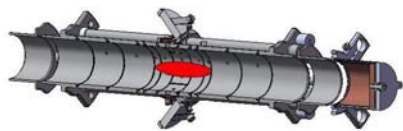
Fig. 2.3: Three-dimensional sketch of the UNIC cylindrical Penning trap.
