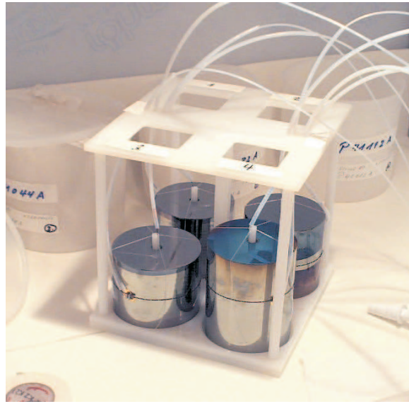
Figure 5.1: The HV and signal cables are connected on the side and central contacts of the diodes, respectively (left). The four first GENIUS-TF bare diodes mounted in the PTFE detector holder (right) [52].
