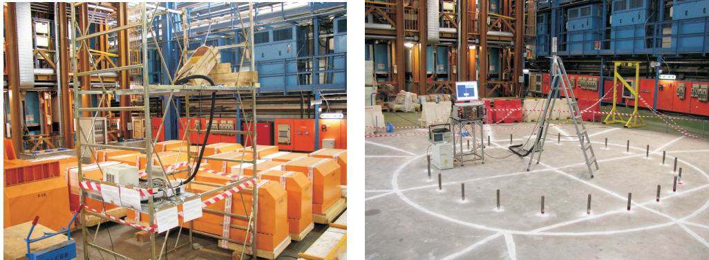
Figure 6.8: Setups for the flux measurements in Hall A in 2004 (left) and 2007 (right). In 2004 the massive parts of the OPERA experiment were stored at the same location as GERDA. In 2007 the flux measurements were performed when the bottom plate of the GERDA water tank was installed.
