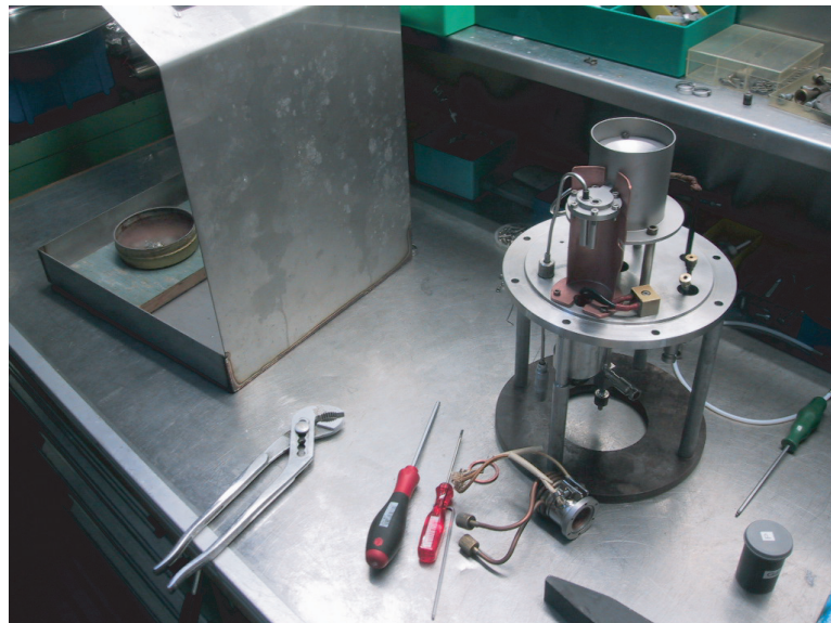
Fig. B.7: (Color.) This MISS is ready for assembly of the cesium reservoir and flanging.
