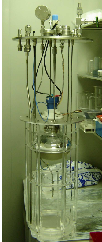
Figure 4.2: The inner part of the LArGe@MPI-K system. From top to bottom: stainless steel lid, aluminium lid, PMT, source-tube and acrylic mounting structure for WLS and diode.
