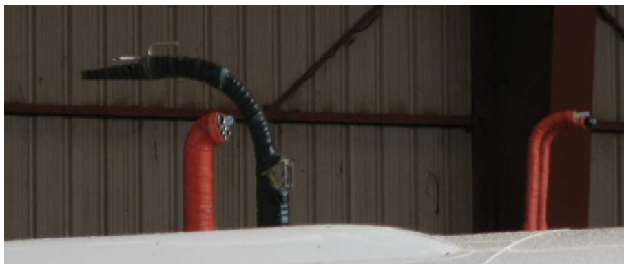
Figure 3.2: The inlet system of the MPI-K CIMS instrument on top of the Falcon research aircraft.
