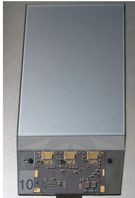
Figure 2.18: Photograph of a one-sensor Inner Tracker module. A pitch adapter connects sensor and front-end chips. The module is equipped with 3 Beetle front-end chips.
