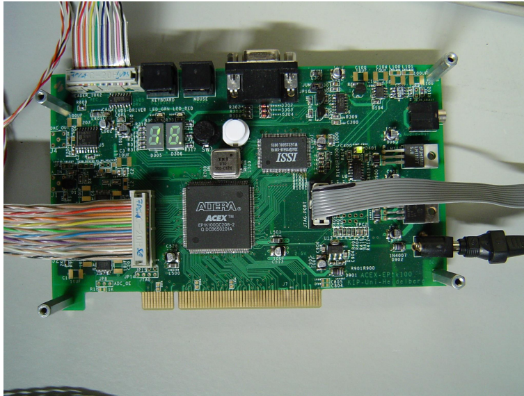
Figure 6.21: Photography of the KIP ACEX board [ACEX]. It is a multi-purpose test board for experiments and exercises, originally designed for lab courses. The card can be used as a standard PCI card in a computer or as a stand-alone device. With two arbitrary external signals the FPGA on the ACEX board generates all digital signals for the random trigger test.
