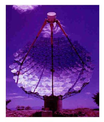
**Fig. 9.** Photograph of the pioneering Whipple imaging atmospheric Cherenkov telescope in Arizona, USA. With a diameter of 10 m it has been until recently the largest operating imaging telescope. The tessellated mirror consists of 248 spherically shaped hexagonally cut mirrors, each 61 cm across. In the focus a fast camera whose pixels are photomultipliers records the shower image against the night sky background (Cawley et al. 1990).
