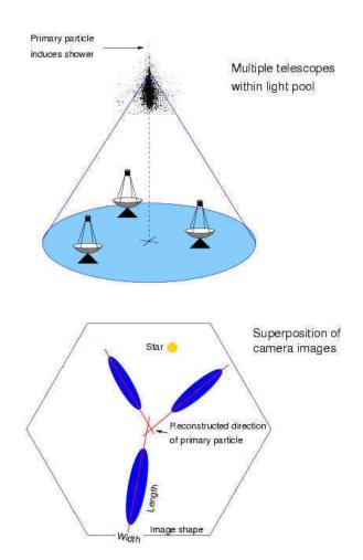
Fig. 10. Stereoscopic  $\gamma$ -ray observation by several telescopes positioned in the Cherenkov cone of an atmospheric shower. The generally elliptical images, superposed into one of the focal plane cameras, determine the arrival direction through the intersection point of their extrapolated major axes. In analogous fashion also the impact point of the shower axis on the ground is determined. This method was first introduced in the HEGRA stereoscopic system.
