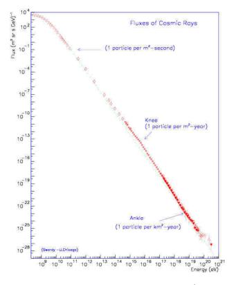
**Fig. 4.** The all-particle CR energy spectrum. For  $E \gtrsim 10$  GeV, the spectrum is a power law, slightly steepening at a few  $10^{15}$  eV, the so-called Knee, and hardening at a few  $10^{18}$  eV, the so-called Ankle. (Adapted from Cronin et al. 1997; courtesy S. Swordy.)
