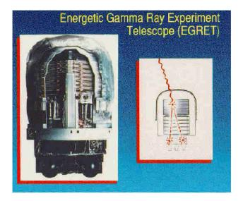
**Fig. 8.** Cut-away of the Energetic Gamma Ray Experiment Telescope (EGRET) on the Compton Gamma Ray Observatory. The track of the pair produced by the interaction of the primary  $\gamma$ -ray in the upper part of the detector is made visible in an adjacent spark chamber (right panel). The detector is surrounded by an anticoincidence hood where, in contrast to  $\gamma$ -rays, charged CRs produce a scintillator signal (left panel).
