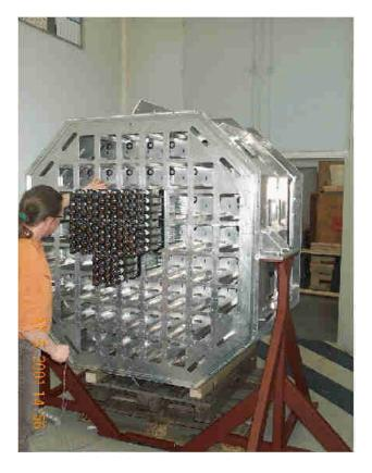
**Fig. 25.** The first H.E.S.S. camera frame at the University VI - VII in Paris, in spring 2001 (with J.-P. Tavernet standing in front). At this stage the camera was partly equipped with photomultipliers and the corresponding electronics in the back. In full configuration the camera has a total number of 980 phototubes (pixels) and a weight of about 860 kg.
