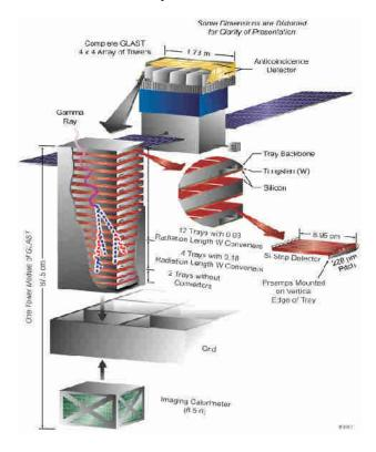
**Fig. 20.** View of the GLAST instrument and its various detectors. The scheme consists of a  $4 \times 4$  array of so-called towers which contain converters for  $\gamma$ -rays together with silicon trackers for the electron/positron pairs, followed by an imaging calorimeter.
