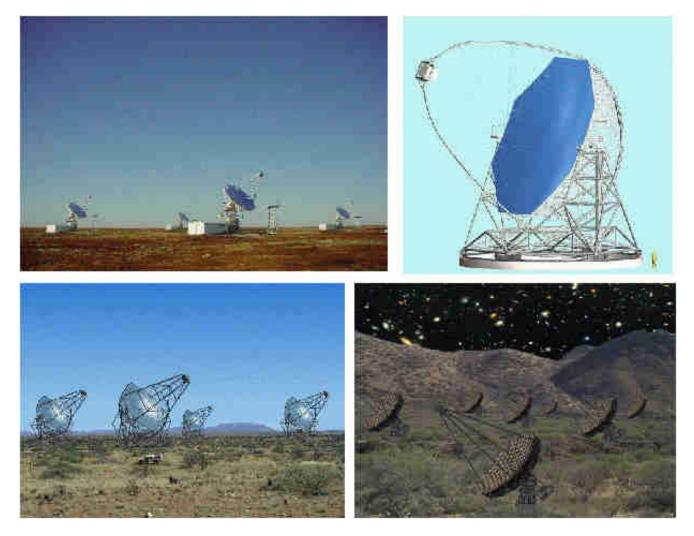
**Fig. 21.** Photomontages/schematics of the main new Cherenkov telescopes. From the upper left to the lower right: the CANGAROO-III system of 4 telescopes (one telescope already in operation), the MAGIC telescope (Major Atmospheric Gamma Imaging Cherenkov telescope), the 4-telescope Phase I of H.E.S.S. (High Energy Stereoscopic System), and the 7-telescope array of VERITAS (Very Energetic Radiation Imaging Telescope Array System).
