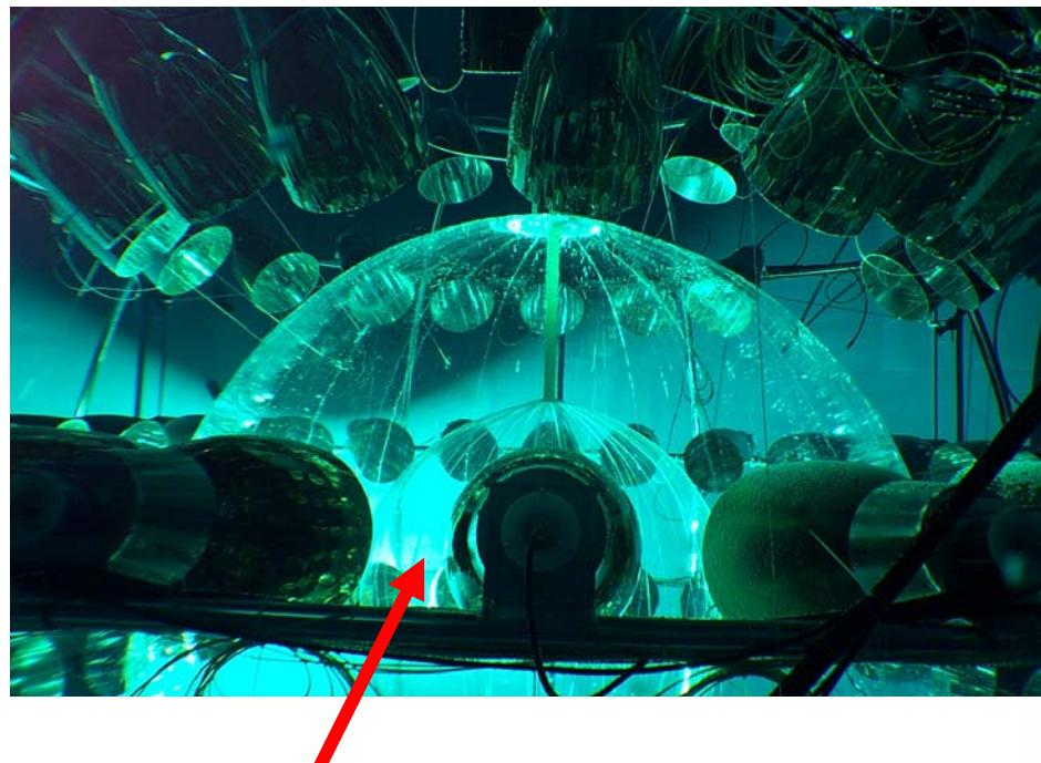
Liquid scintillator target
