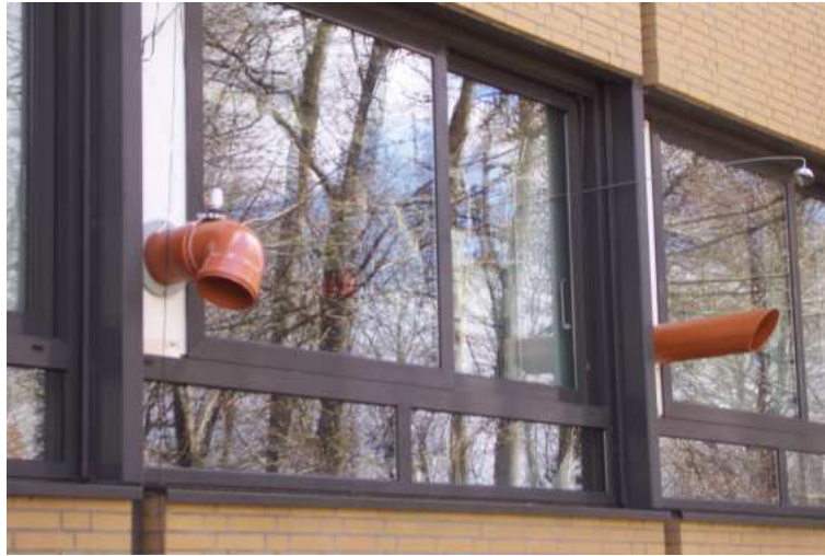
Figure C.1: Photograph of inlet and exhaust (only atmospheric air) system. (The measurement exhaust was filtered via the exhaust system of the MPI.)
