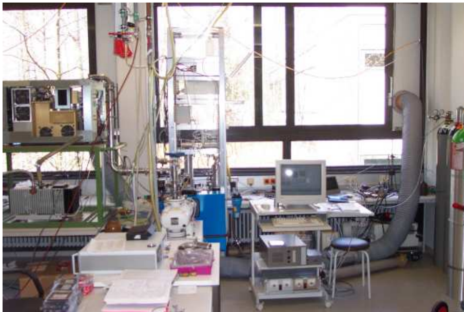
Figure C.2: Photograph of complete setup: PITMAS (left), DMPS (middle), exhaust (right).
