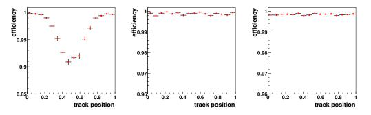
Figure 4: Efficiency versus track impact position for IT3 (left), Glast2000 (middle) and CMS (right).
