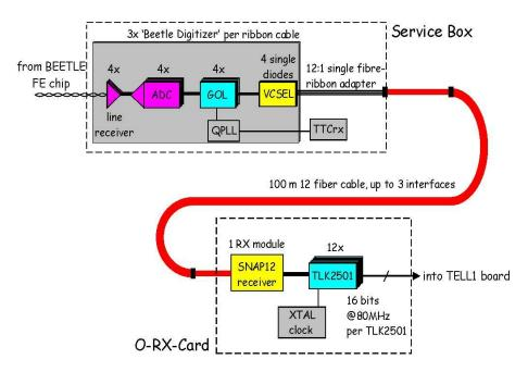
Figure 5: Sketch of the digital optical readout link.
