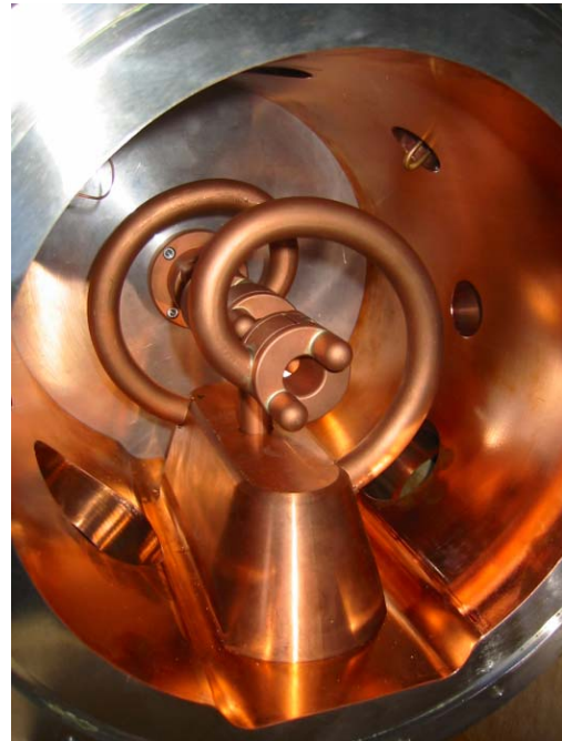
Figure 1: View of the spiral loaded cavity with finger drift tubes.
