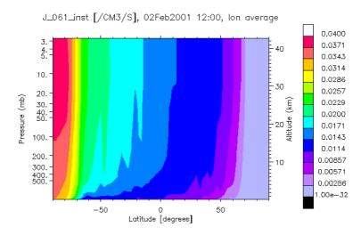
Figure 2.3: Photolysis rates  $(s^{-1})$  for  $Br_2$  in MOZART4. Instantaneous output.
