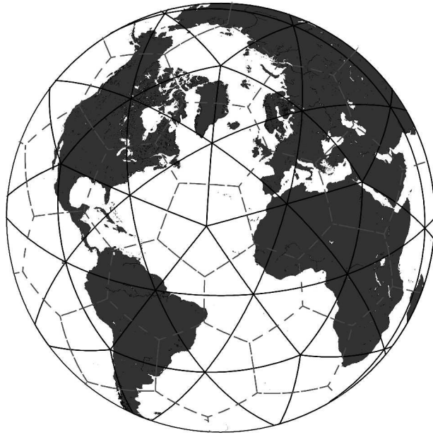
FIG. 1. Delaunay (triangular) and Voronoi (hexagonal-pentagonal) icosahedral grid at the first grid-refinement level.
