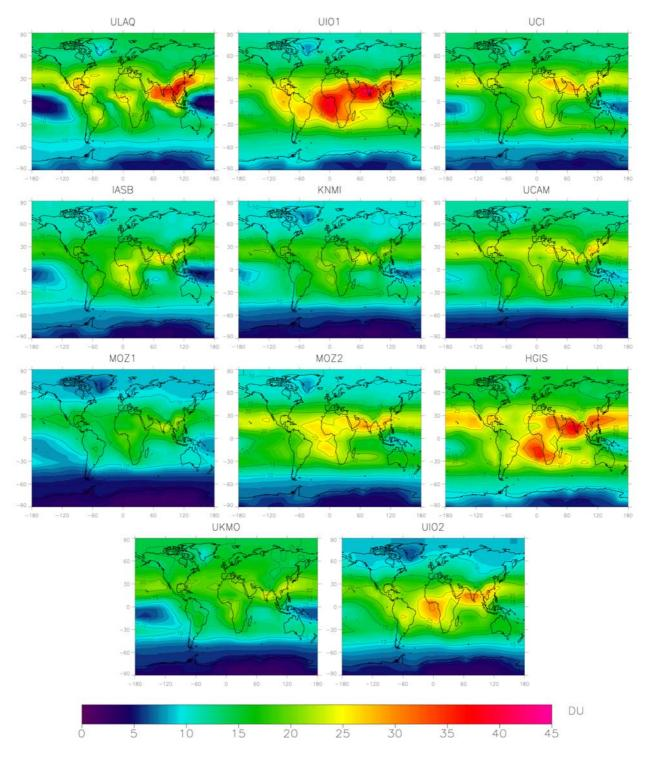
**Figure 3.** Change in the annual mean tropospheric ozone column from 2000 to 2100 (DU). The tropopause level in this calculation is based on the temperature gradient as described by *Berntsen et al.* [1997].
