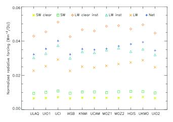
**Figure 8.** Normalized global mean radiative forcing due to changes in tropospheric ozone between 2000 and 2100 (W  $m^{-2} DU^{-1}$ ), separated into shortwave (SW) and longwave (LW) components and calculated under different assumptions. Clear, clear-sky conditions; inst, no stratospheric temperature adjustment; and net, LW + SW.
