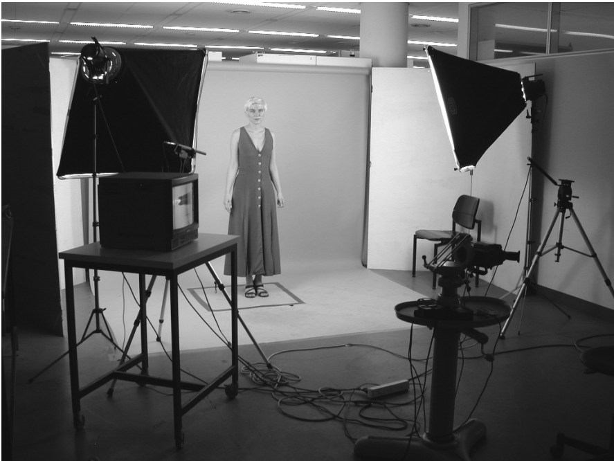
Fig. 2: Setup for videotaping dance motions.
