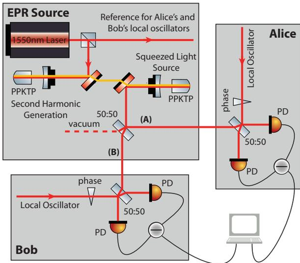
Figure 1: (Color online) Schematic of the experiment. A continuous-wave laser beam at 1550 nm (red) was frequency doubled (yellow) and used to produce squeezed light at the fundamental wavelength via type I parametric down-conversion. A balanced beam splitter subsequently mixed the squeezed light with a vacuum mode. Amplitude and phase quadrature amplitude measurements on the output beams by means of balanced homodyne detectors proved EPR entanglement amongst them. PD: photo diode.
