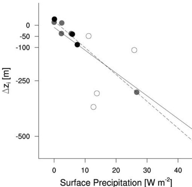
**Figure 12.** Difference in the final depth of the marine layer between the precipitating and non-precipitating simulation for each model as a function of the rate of precipitation in the precipitating simulation. Regression lines show best fit for all simulations (solid) and only the bin and two-moment schemes (dashed).
