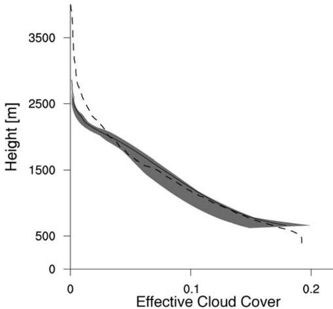
**Figure 7.** Lidar and effective LES cloud cover. The lidar cloud cover, shown by the dashed line, is the cumulative cloud cover and must monotonically increase as one traverses the layer (from top to bottom). The total cloud cover is given by the cloud fraction at cloud base. For LES the effective cloud cover is reconstructed from cloud fraction versus height data, and scaled to match the lidar near cloud base. The shaded area denotes the interquartile difference, as in Fig. 3.
