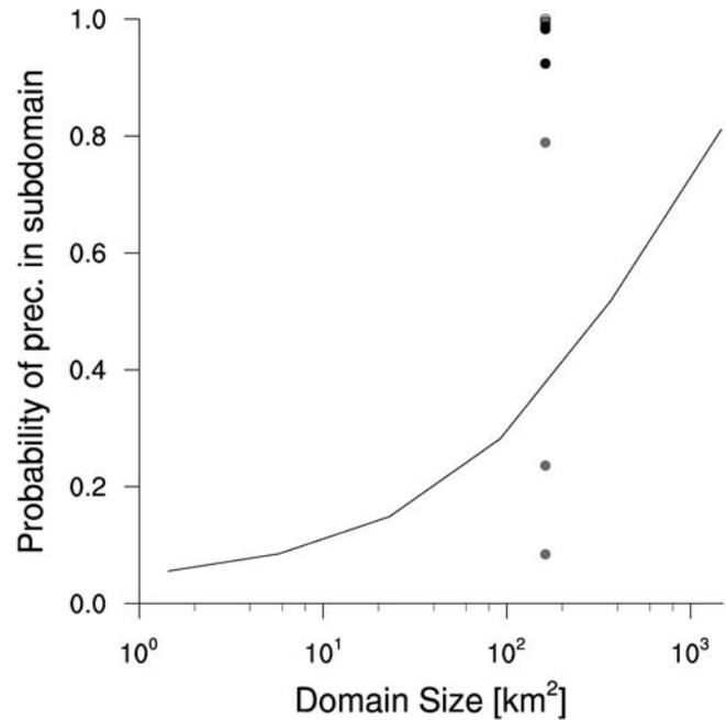
**Figure 10.** Probability of precipitation in subdomains of size  $\ell$ . Circles show the LES data, with symbols as in Fig. 9. Almost all the points, except for three of the two-moment simulations, group under the black dots near a probability of unity, indicating that precipitation was almost always present in the LES.
