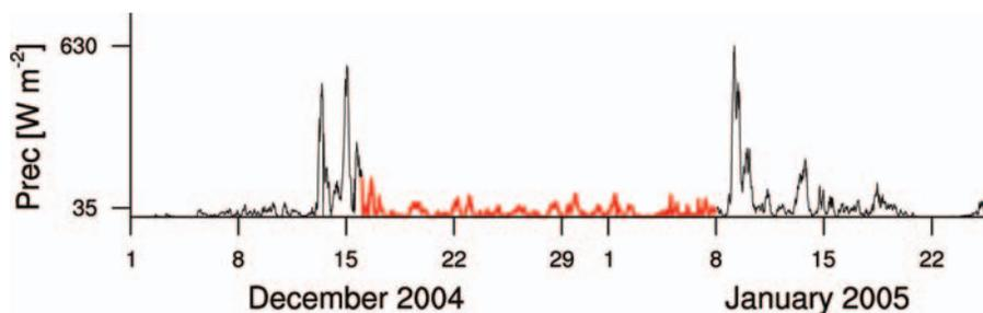
**Figure 1.** Area averaged precipitation for each S-pol radar ( $0.5^\circ$ ) surveillance scan plotted for the months of December 2004 and January 2005. The thick red line indicates what we refer to as the undisturbed period over which we composite (see text). Ordinate values denote the maximum and average precipitation for the entire period.
