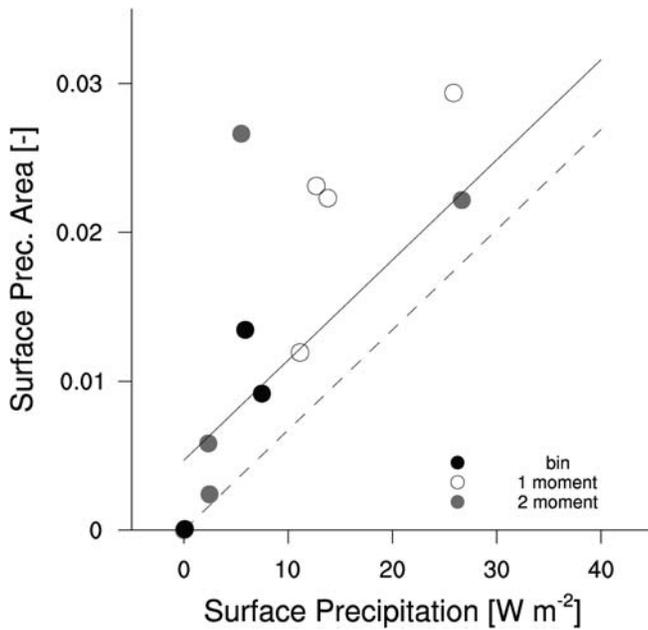
**Figure 9.** Raining area as a function of net surface rain-rate, with dots denoting the different models and the lines denoting the radar observations, with reflectivity to rain-rate being converted using either the TRMM (solid line) rain -rate reflectivity relationship. The dashed line has the same slope as the solid line but with no offset.
